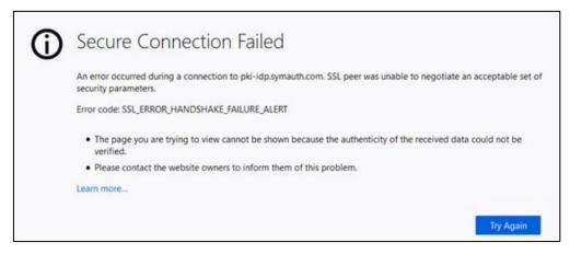
This can be resolved by navigating to the settings of the Security Devices for PKI Client. From the **Open Menu** panel select -> **Options** -> type "Certificate" in **Find in Options** text field -> click on **Security Devices** button, and
